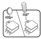
Replace the battery cover and tighten the screw to secure the battery cover.
